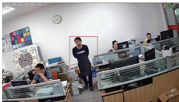
3. How to enable the AI playback function: First, the camera needs to support the AI function (humanbody or humanface); after the NVR enables recording (Time type or Motion type) and the camera enables the AI function, each AI type alarm event will generate a zoom Thumbnails, click on these thumbnails to directly play back the video when the event happened.
