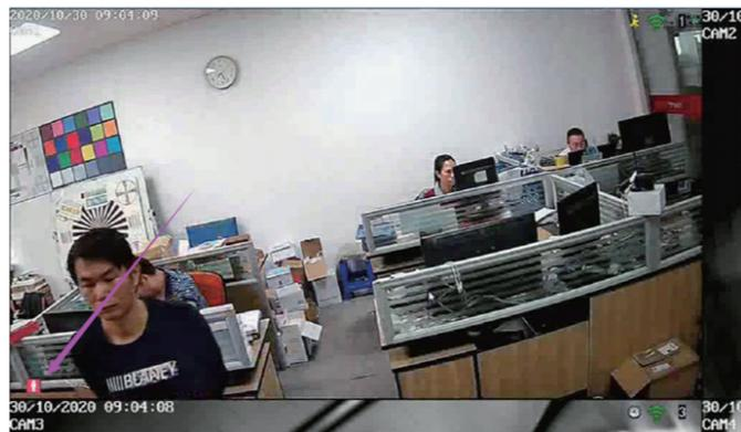
2. How to enable the Bodyregion function: Check the Bodyregion option and click "Apply" to enable the Bodyregion function (each channel also needs to be set independently). When a humanoid image is detected on the screen, the NVR will use a red frame to mark the position of the humanoid.
